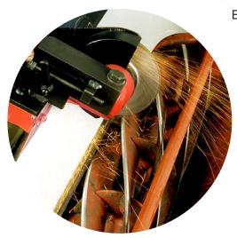
Before the relief on your reel is completely lost, you can restore it in minutes with this handy machine. Portable and fast, it saves putting your unit onto a grinder.
