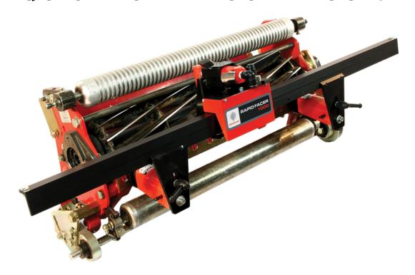
Its unique bar aligns an accurate face on the bedknife in just 90 seconds.
