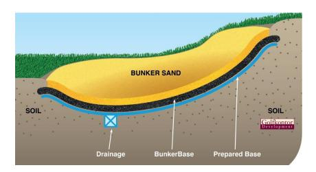
Polylast, a highly porous material made from recycled rubber, promises revolutionary relief in bunker care: in heavy rainfall it allows water to flow through freely at any point of impact, while preserving the sand above from erosion and dirt from the native surface. The liner comes with a 10-year warranty!
